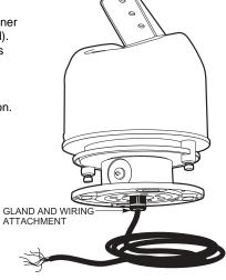
Figure 2. Bottom View, Wire Attachment
